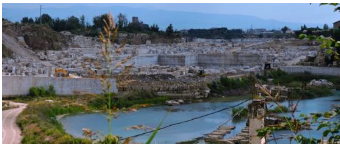
Travertine quarry in Tivoli. Most of Roman buildings were built with this stione, from Roman temples to University Campus
